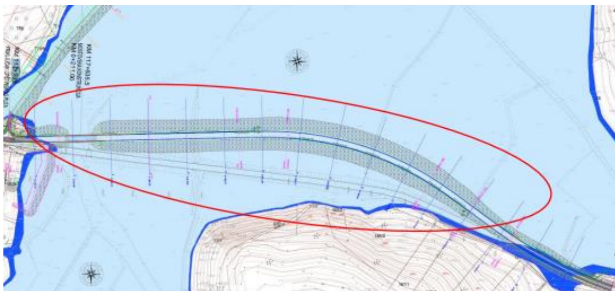
Figure 8 Location of the old and new alignment of the State Road IB-21 (Source: Conceptual Design for the State Road IB No.21)
